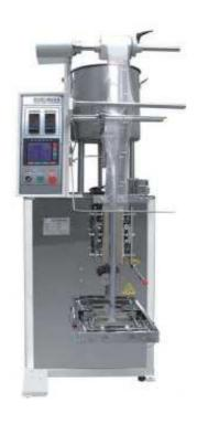
The machine is suitable for small doses of jelly, liquid.
