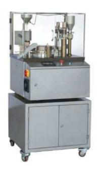
SED-120J Fully Automatic Capsule Filling Machine is used to fill powder, grain, and tablet. It adopts multi-bore dosing, intermittent motion and timing frequency conversion.
