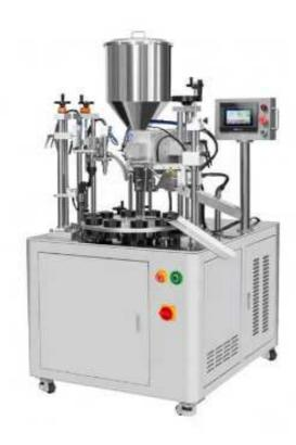
Packry's HX-006 Plastic Tube Filling and Sealing Machine, it's the type of high-speed aluminum Plastic tube filling and sealing machine which is widely used for closing cream lotion tube cleanser moisturizing and medicine hose.
