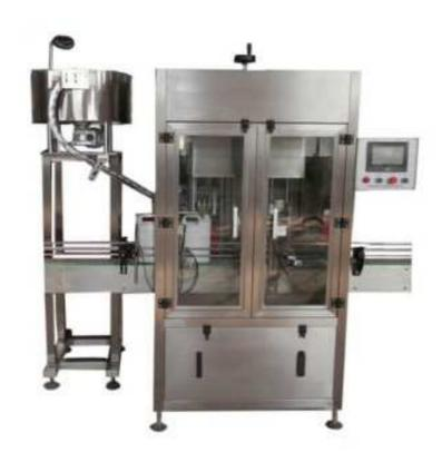
This machine integrates machinery, electricity, gas into integration, is the new high-tech product. The man-machine interface system, it is convenient and swift to adjust the specification. The machine is made up with cap scrambler, cap suppliers, cap scraping and cap screwing which is suitable for automatic capping for large buckets.
