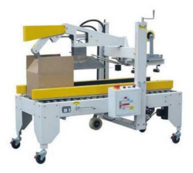
Auto folding for top lid ensures smooth and suitable sealing motions. The entire sealing operation is automatically performed, providing elegant outlook and labor-saving, the machine can be operated together with automatic packaging line.
