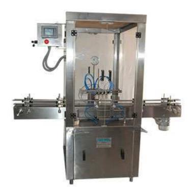
Automatic Vertical Air Jet Cleaning Machine works on positive air pressure & vacuum cleaning. The unit is made compact, versatile and enclosed in stainless steel elegantly matt finish body, consists of S. S. Slat Conveyor & Reciprocating cleaning nozzles. No container No cleaning system arrangement is standard features of the machine. The main drive of the machine and conveyor drive consists of A/C Motor with synchronized variable A/C Frequency Drive.
