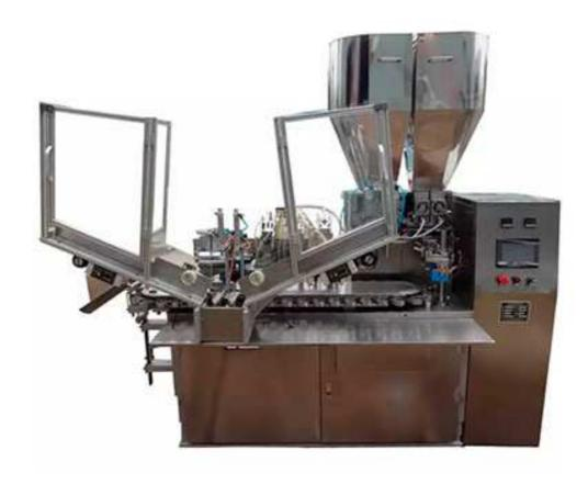
The HTGF-100 automatic tube filler tube sealer is suitable for filling all kinds of semi-viscous and viscous products into plastic or metal tubes. It can be used for pharmaceuticals, food products, cosmetics, and chemicals. Some of the products filled with this tube filler are ointments, lotions, caulks, adhesives, cheese spreads, and peanut butter. This tube filler/sealers offers quick adjustment, which makes it suitable for using multiple types of soft plastic and/or metal tubes.
