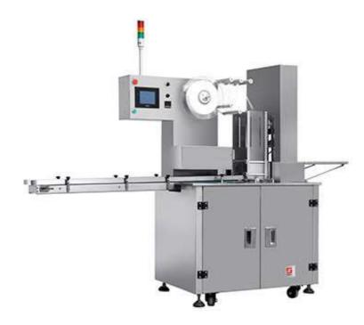
The machine adopts PE film tapes to carry out automatic counting, palletizing and baling of many pieces of objects so as to save materials and energy to the utmost extent. It is widely used for automatic assembly packaging of many pieces of objects in medicines, food, stationery commodities and other industries, and especially has wide application in injections of the pharmaceutical industry.
