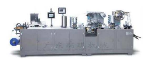
The tropical (AL/PL/AL) pharmacy blister packaging machine is invented on the basis of national-level key new products. It can be used for three different kinds of packaging: AL/PL, AL/AL, AL/PL/AL, up to the purpose of one machine three uses.
