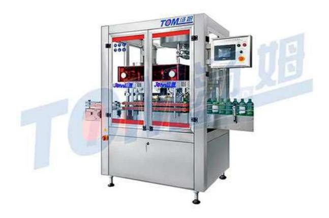
This capping machine perfectly used for diversified containers in different materials and shapes, such as plastic bottle, glass bottle, metal bottle, etc. caps or bottles changeovers are very quick, easy to be performed. No bottle no capping during the machine cycle. Conveyor, capping machine and bottle clamping belt can separately frequency conversion applicable for allowed various capping range. Meets GMP standard, protecting door may optional which guarantees more safe and environmental.
