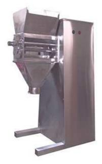
The machine is special equipment. Under the action of barrel through clockwise and counterclockwise rotation, the machine can make mixture of damp powder pass through forcibly sieve to become granule. The machine is mainly suitable for granulating granule with different specification in pharmaceutical industry, chemical industry, foodstuff industry etc. After dried by baking, press the granule to all kinds of shaped product.
