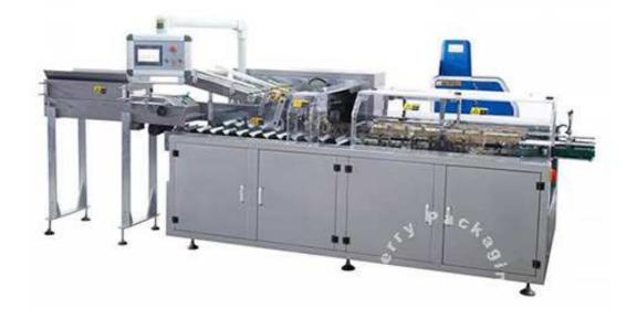
This machine is suitable for packing blisters, tubes ampoules and other related objeces into boxes intermittently. The higjest speed can up to 150boxes/min. It has advantage of high packing efficiency and good quality. This machine can fold leafiest, open box, insert blister into box, emboss batch number and close box automatically. It adopts inverter to adjust speed, human machine interface to operate, PLC to control. and photoelectric to monitor and control each
