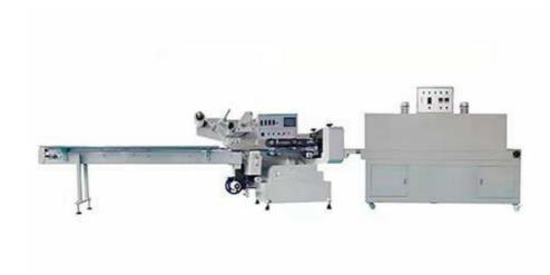
It works from feeding, bag forming to sealing and shrink wrapping, widely used in food, medical, cosmetic and stationery industry.
