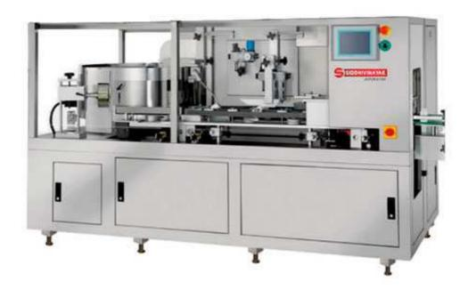
Bottle Unscrambler - SVAHBU Bottle Unscrambler is designed to provide a loading solution for empty containers and delivers them to the downstream equipment conveyor in vertical condition lines in a controlled and repeatable manner.
