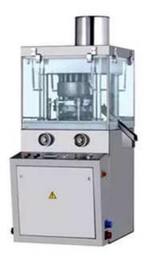
ZP11/ZP18 Rotary Tablet Press is used in electronic industry, food industry, chemical industry, articles of everyday use industry and pharmaceutical industry, for pressing various granular raw materials into special shaped tablets. Such as electronic element, camphor ball, catalyst and powder metallurgy.
