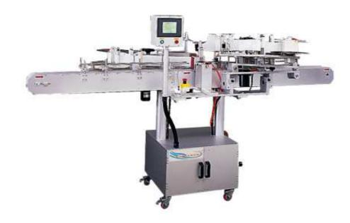
Specially used in labeling the barrel and bottle neck of tubular objects.
