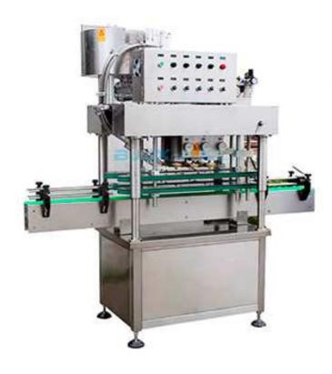
This machine is a universal capping machine. When bottle, cap is changed, it needn't change parts, having high cap-revolving qualification, high speed. The bedding cover part adopts photoelectric control, improve the speed for cover.
