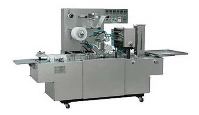
The three-dimensional packaging machine 3D WRAPPING MACHINE is designed for the packaging of cigarette boxes. It has a full set of functions of automatic feeding, stacking, packaging, heat sealing, sorting, and counting, and can realize single or multiple integrated packaging of boxed products.
