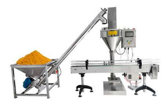
This machine is easy to operate by PLC touch screen. It is mainly suitable for packing powdery and micro powdery materials, such as flour, sugar, xylitol, milk powder, pesticide, veterinary medicine, dye, chemical agent, food seasoning, additive, enzyme preparation, etc.
