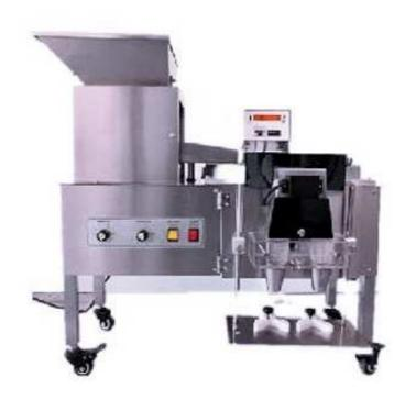
This machine has been designed and developed to count & fill different shapes or size of products accurately like soft gel capsules, hard capsules, tablets, sugar coating, and film coating tablets, pills, herb medicine or similar products into containers or vials.
