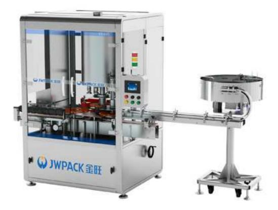
The capping machine combines bottle input, cap unscrambler, capping and bottle output together, it is positioning capping. The machine is rotary structure, it will not damage the bottle and cap during operation and has the features of high capping qualification rate, stable operation and wide application. It is used for capping of different sizes of glass and plastic bottles. The machine is controlled by PLC, touch screen and easy operation.
