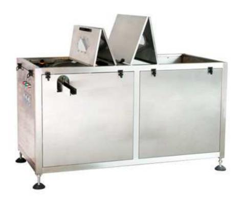
SLP-X series round bottle unscrambler can sort round bottles automatically and put the containers stand on conveyor with high speed. The unscrambler consists of main sorting unit, cover with door, and bottle feeding system with storage tank. It is easy to operate and stable running and widely used in the pharmacy, food & beverage, cosmetic & personal care industries.
