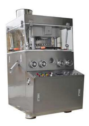
This machine is a continuous automatic tablet press for pressing granular raw materials into tablets. It is mainly used in pharmaceutical industry and also the chemical, food, electronic, plastic and metallurgical industries.
