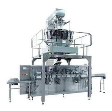
Automatic bag feeding particle packaging machine adopts Germany's Siemens PLC control, with touch panel human computer interface control system. It is easy for operating.
