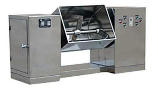
CH type mixer is widely used for mixing powder or wet raw materials and can make the main and auxiliary raw materials with different proportion uniform.
