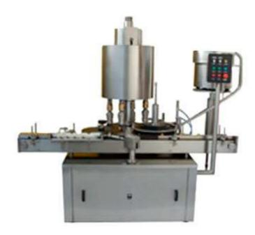
Automatic Multi Head Screw cap sealing machine is versatile, self-supported on stainless steel leg with height adjustable adjustment system. The machine is precision built on sturdy welded steel frame completely enclose in stainless steel sheet and doors are provided to facilitate the servicing of machine.
