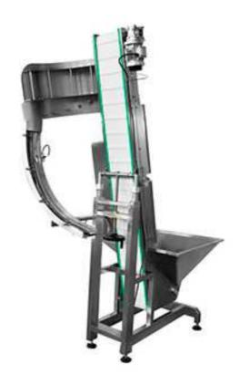
The CapperPacks Cap Sorting Elevator is suitable for threaded round caps. Manually pour the caps into the bucket of the cap elevator, and the machine automatically sorts and lifts the caps. The caps are moved from the slide rail to the cap hanger. With the cap rubbing machine, there is no need for spare parts when replacing the caps, and only need to operate the hand wheel to adjust slightly to meet production requirements.
