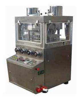
This machine is a double-press type; it continually and automatically tablet press granular raw materials into round tablet, irregular tablet, carved tablet and two layer (color) tablets etc. It is mainly used in pharmaceutical industry and also the chemical, food, electronic industry and so on.
