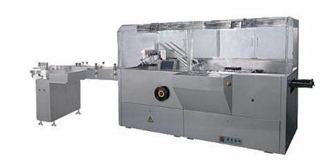
This machine is suitable for cardboard case packaging of bottles (round, square), cosmetic, food and so on. It consists of direction folding (1-4 folds) and feeding equipment, cardboard case forming and feeding, batch number printing, sealing of case tongues at both ends etc. The whole encasing process is finished automatically. It can be added hot-glue machine.
