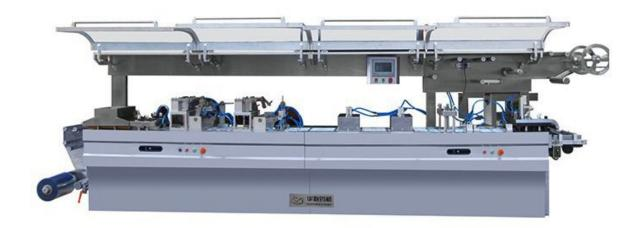
This machine is suitable for automatic high speed alu pvc packing of capsules, tablets and other regular shape medicine. It adopts flat pressure forming to form strong and average blisters, and roller type mesh sealing to ensure reliable sealing. The machine is equipped with batching system, embossing device and horizontal boundless punching to achieve high automation and efficiency.
