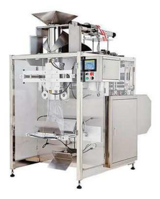
TD-V35L VFFS Packaging Machine for Liquid uses servo-driven film roll. Color touch screen operator interface, tracking automatically adjust depending on length of the bag packaging film printing position.
