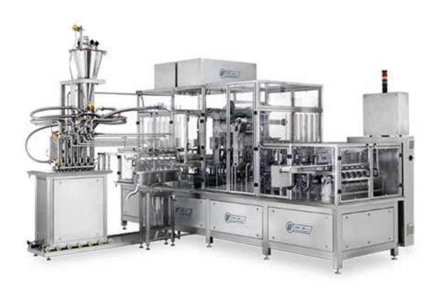
PXM is a fully automatic, in-line filling and sealing machine that is based on digital, mechanical and pneumatic assemblies. This automatic packing machine is suitable for packaging a wide range of liquid, paste, granulated and powdered products into preformed containers of various size and shapes. The machine can be used for dairy products, salads, dressings, desserts, dry soups, frozen dishes, cosmetics and much more.
