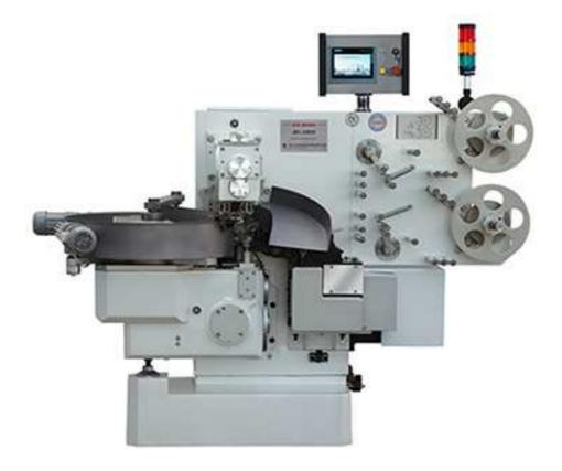
Wrapping machine for hard candies in double twist wrap. The machine is suitable to wrap diesformed or deposited sweets of round, oval or oblong shapes. Sweets with semi-liquid centers can be handled without problems. The JH-S800 is able to be equipped with a sorting station to eliminate sugar dust, chips and broken pieces. An efficient feeding is achieved by the approved plate feeding system. The machine is provided for the use of one wrapping material.
