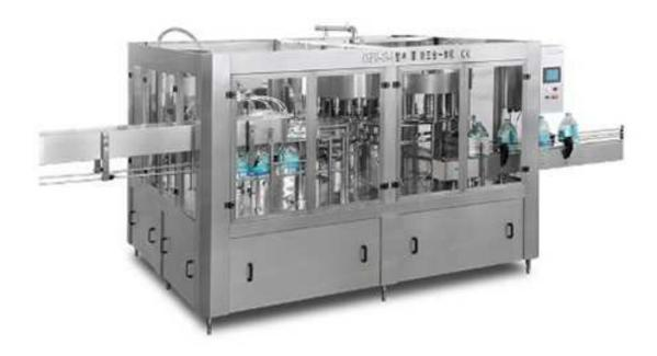
The washing, filling, packing is integrated into this car. The machine is suitable for bottling water in PET bottles in the mode of gravity filling. Each element of the machine, which is in contact with the liquid, is made of high quality stainless steel. The production capacity is 4000-24000 bottles per hour.
