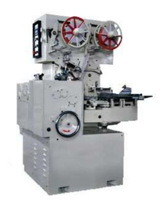
BF500 Cut and Wrap Machine is used for packing a wide variety of confectionery products, like chewy candies, toffee, gum, Bun, caramel, Milk-candy, Soft Caramel etc. The machine produces a perfect cut & wrapped product, square, oblong, cube, log shape. The maximum running speed is 500 wraps per minute, the machine as standard is fitted with an optical print registration unit. The machine is full variable in speed. The machine wraps in double twist wrap style.
