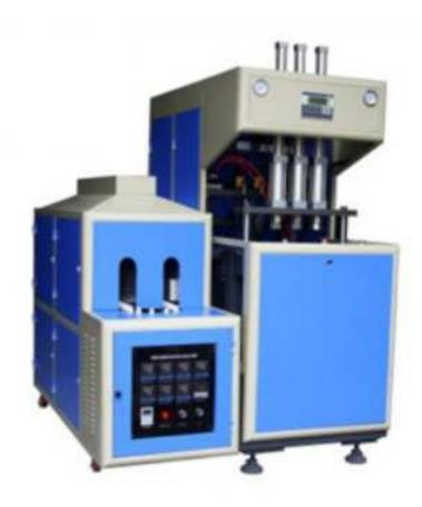
ES-B3 two step manually preform inserted full auto bottle blower is applicable for blowing the carbonic acid beverage bottle mineral spring water bottle, farm chemical bottle, oil bottle, medical, hot-filled bottle in any shapes and made of PET raw material.
