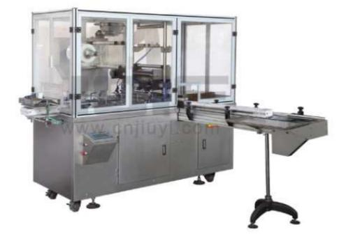
The machine is driven by a series of cams, connecting rods and other accessories, which are applicable for wrapping big-sized cases such as multi-boxes, which driving principle is intermittent. Model JE-400C overwrapping machine is applicable for wrapping big sized box such as food box with biscuit/chocolate etc. using BOPP film with tear tape.
