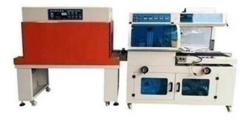
L type shrink packaging machine which uses roll-fed thermoplastic film folded in half along its length. A product or group of products are placed between the two halves of film. The film is then sealed and cut off around the product with an L shaped sealing bar. The pack is then passed through a heated tunnel to shrink the film around the product to produce a tightly enclosed pack. Widely used for wrapping books, video tapes, floppy disks, foodstuffs such as dried fish, boxed products, etc.
