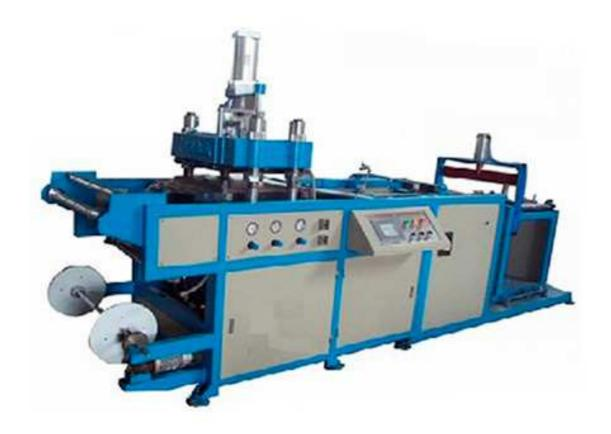
It is suitable for thermoforming BOPS, HIPS, PP, PET PVC, PS, sheet that can produce varieties of blister package and blister tray. For example: curatorial injection tray, oral liquid tray, mobile telephone tray, cookies tray, one-off tableware etc..
