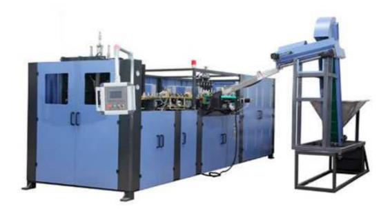
SD-LG Series fully automatic bottles blowing machine is one of our most stable two-step bottles blowing producing equipment. Its producing range is mainly for the CSD bottles, drinking water bottles, other beverage bottles, and chemical or pharmaceutic bottles, it can blow maximum 750ml bottles, largest producing capacity reaches 5000 bottles per hour.
