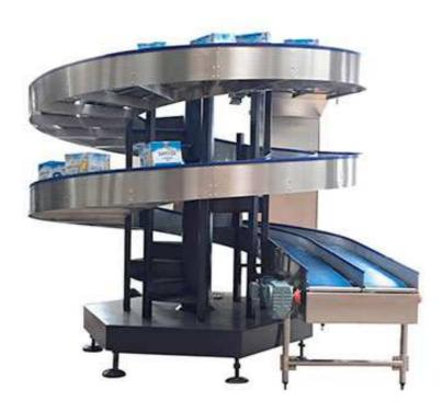
This chain plate spiral conveying machine is widely used to lift and convey products in such industries as food, beverage, chemical industry, etc. Compared with other types of lifter, it has such features as saving floor space of conveyor machine, continuous conveying, etc.
