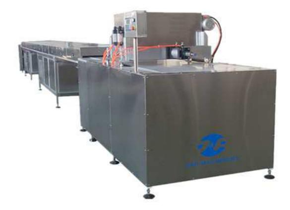
The chocolate chip depositing machine can produce smallest 0.098g chocolate chips and big chocolate drops. The depositor can be pneumatic or servo motors. There is a cooling tunnel to cool down chocolate chips. The width of the conveyor belt can be from 600mm to 1200mm.
