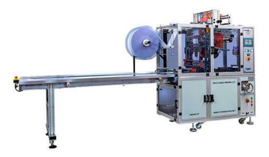
An idal machine for over-wrappering & Bundling Soap Bars, Biscuits, Waffle Box Multi-packs. This machine is feed manually by one or two operators. Also a special design with full automatic feeding system connected directly to the production line is ails available depends on the way of production output. AW2003 - FF Machines have Mechanical and easy OOP Lneght adjustment & Change - Over features. Optionally, elevator system can be provşded for 2 rows of stacked packaging.
