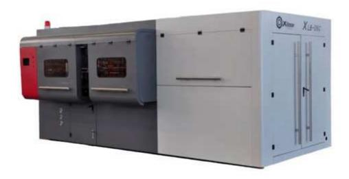
The 4000BPH 5L Blowing Machine is equipped with advanced oil-free airbag clamping technology, the clamping force is large, and the toggle operation has less force and long life. Due to the high and reliable performance, it realizes the function to ensure that the blowing method is fast, high efficiency, good quality and so on.
