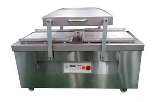
This model has two independent vacuum chambers, while the vacuum chamber is placed on the package while the vacuum chamber on the other side is being vacuum packed, so the packing speed is doubled.
