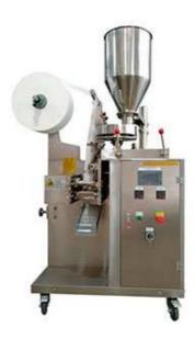
This machine can automatically complete bag-making, filling, measuring, sealing, thread feeding, tag attaching, cutting and counting, etc. It would highly inporve the working efficiency and reduce labor expenses.
