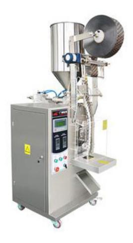
The MK-60YB Vertical form fill seal machine uses a liquid filler as the weighing device, applicable to the packaging of liquids, pasty liquids and sauces. A stirrer and heater can be added to fully mix the materials for full melting and better flowability, ensuring smooth downstream filling and packaging operations without wire drawing.
